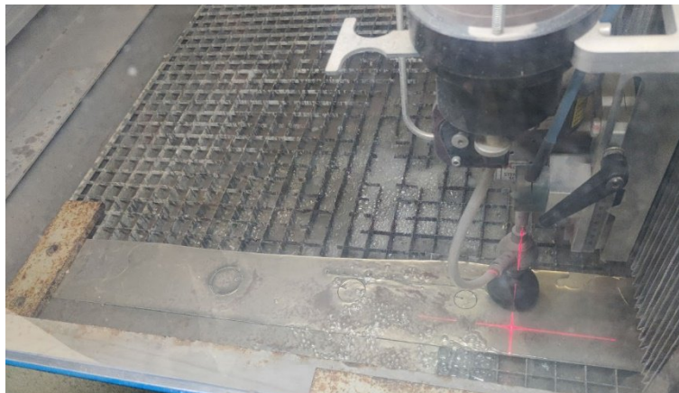
Water-jet cutting process, resulted from the CAD
